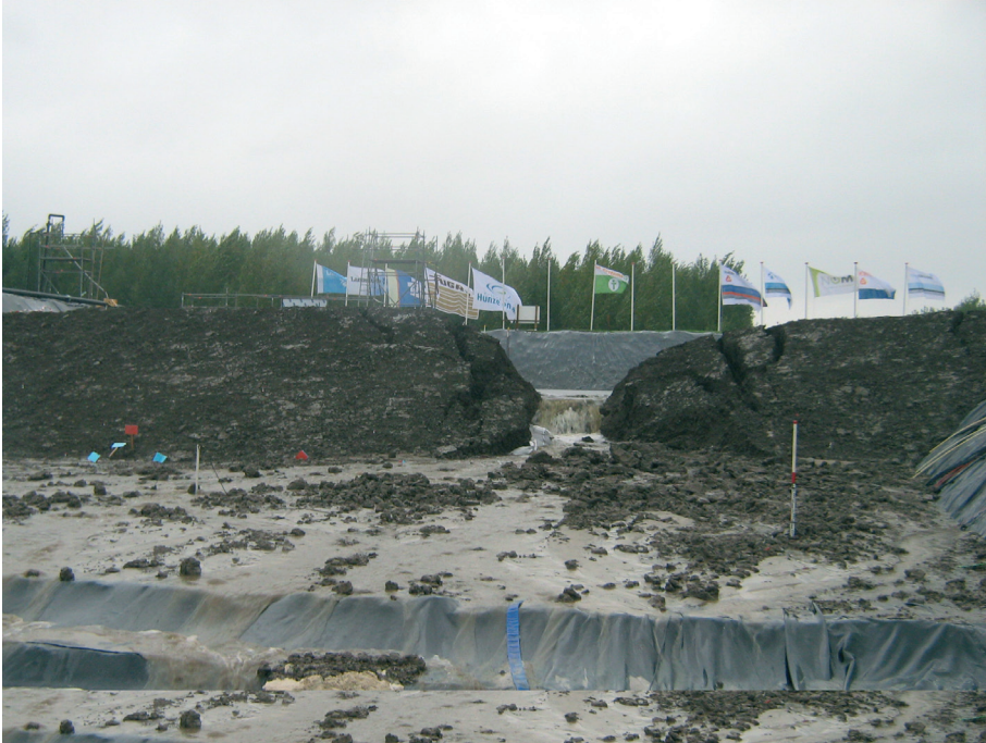
Figure 4.6 An Ijkdijk after an experiment in late 2009. Photo by Vera van Beek. © Deltares.
