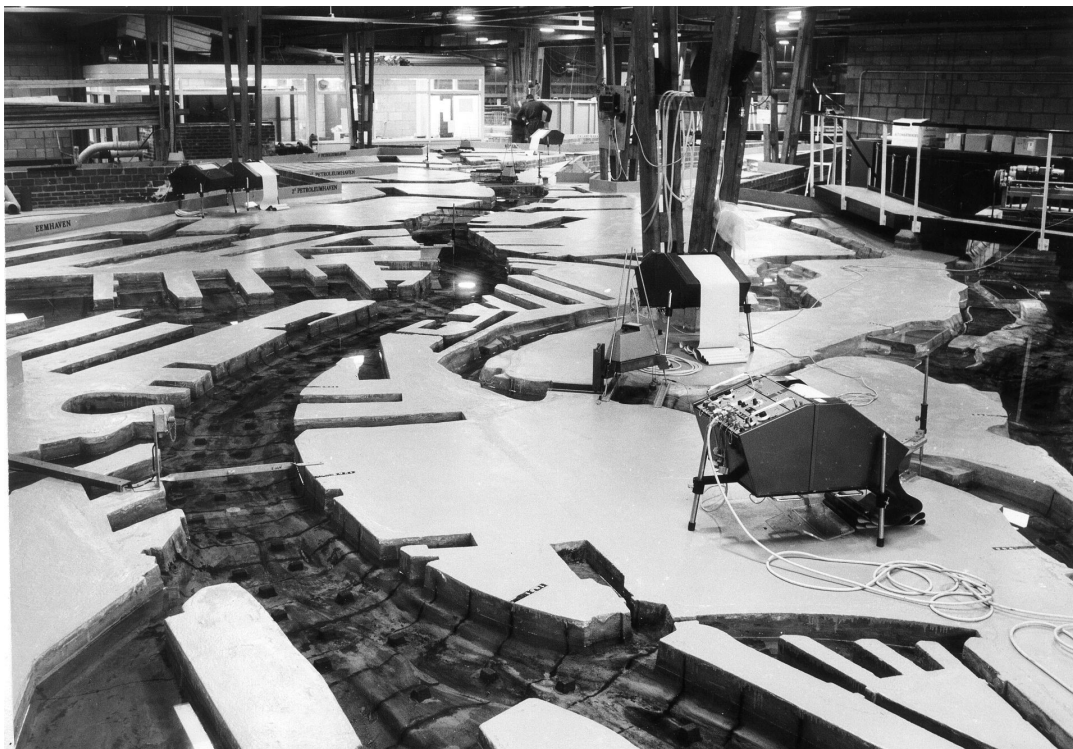
Figure 2: A scale model of the Rotterdam harbour and hinterland in operation. Note the devices used to register water levels located at various points of the model. © Deltares.
